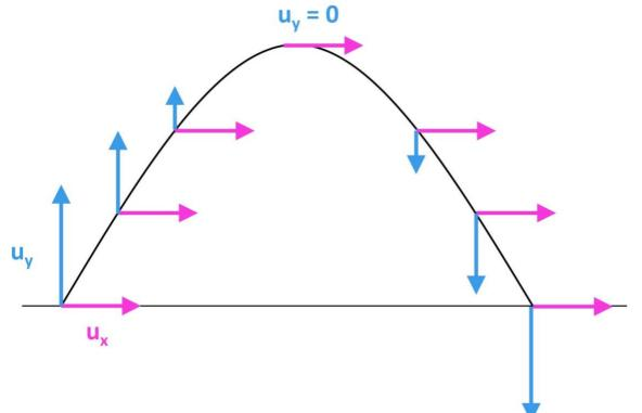
When modelling projectile motion problems, the horizontal and vertical vector components are analysed separately. The diagram below illustrates how the initial velocity, *u*, is resolved into its horizontal and vertical components:
