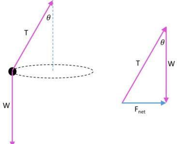
The triangle that forms as a result of  $F_c$ , W and T can be used to analyse lengths/distances and forces by applying trigonometry.
