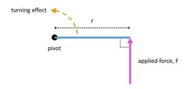
Often, the force is not applied at right angles and in these situations, it is only the component of the force that is perpendicular to the line between the pivot and the applied force that results in torque.
