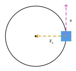
One of the features of circular motion, is that the centripetal force is always directed into the centre of the circle that is the path for the object. Even though the object is constantly changing direction, the motion at any instant is always tangential to the circle. This gives us the situation where the angle,  $\theta$ , between the force and the direction of motion is 90°. If we apply this to our equation for work:
