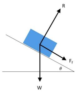
The diagrams break down the weight force, the normal reaction force and the friction force into horizontal and vertical components:
